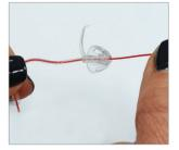
3. Carefully push the cleaning tool through the dome past the vent without removing the dome.
