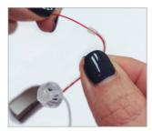
2. Insert the cleaning tool into the top part of the tube and feed it all the way through to the dome.
