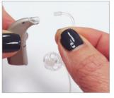
1. Detach the corda tube by pulling the tube away from the hearing instrument.
